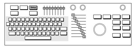
After exiting Setup, you can save the settings by touching the **Save Preset** control (located in the lower left corner of the left touch panel).
