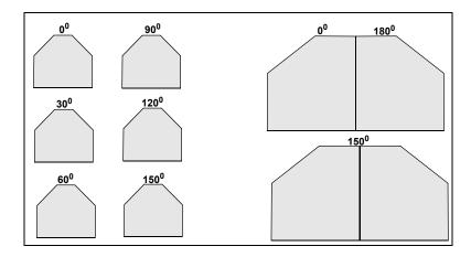
The first and last images acquired should line up, as if they were a single image. Use this comparison mode to determine if you need to do another acquisition. Fig. 1 shows an example where the first and last images line up correctly at 0 and 180 degrees. Fig. 2 shows an example where the images do not line up and another acquisition should be considered.
