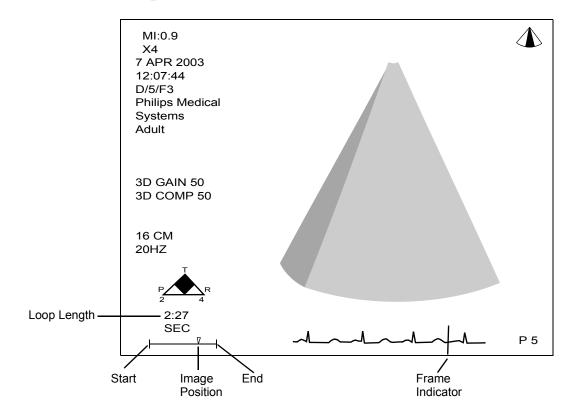
The following illustration shows the controls that are used in Live 3D Loop Display mode.
