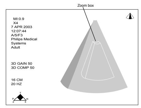
2 On entering 3D Preview mode, the **Position** control is highlighted, and you can use the trackball to move the zoom box to the region of interest by moving it up and down or side to side.
