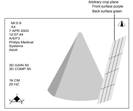
2 Using the trackball, move the crop plane vertically and horizontally around the rendered image.
