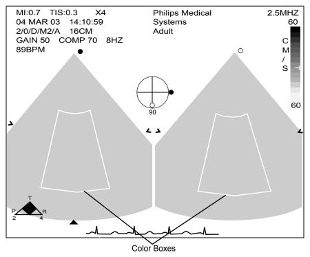
In lateral tilt and rotation modes, the box on the right image tracks the left color box vertically, but does not move left or right because the color boxes together define a contiguous color volume. In elevation tilt, however, the boxes in both images move together.
