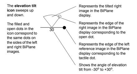
**NOTE** Both elevation tilt image planes are at 0<sup>o</sup> rotation.
